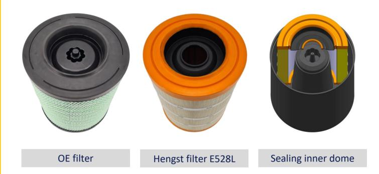
In the end disc of the Hengst filter is a recess in the place where the key-lock system of the OE filter is located. In addition, a sealing contour has been added to the top of the filter, which is compressed when the cover is closed to ensure the proper function of the filter.
