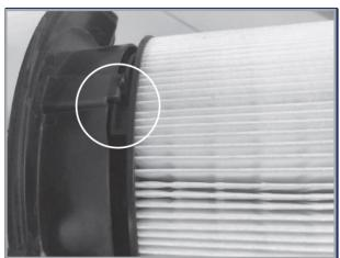
Make sure that the locking of the filter is correct on all 3 positions
