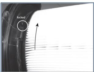
Make sure that the locking of the filter is correct on all 3 positions
