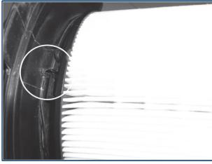
Push the filter firmly and rotate clockwise until locking pin clicks
